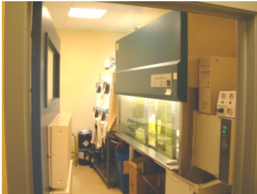
Figure 2: The 'alpha-lab' with a closed-circuit of the glove box, Biohazard and the incubator.
