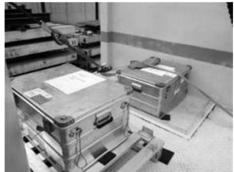
Securing packages in the loading area (stowage)
