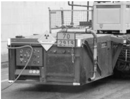
TN17T at Tihange: UN 2919 = special arrangement, packaging empty
