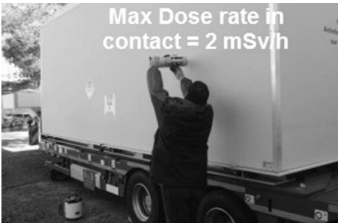
Figure 3 – Maximum dose rate permitted on the surface / in contact of the vehicle
