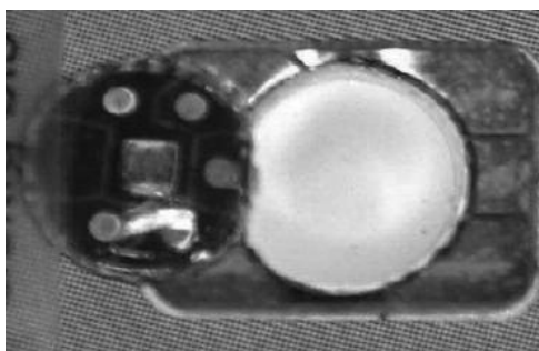
Figure 2: The chip is surrounded by an epoxy encapsulant, responsible for the OSL signal [8].
