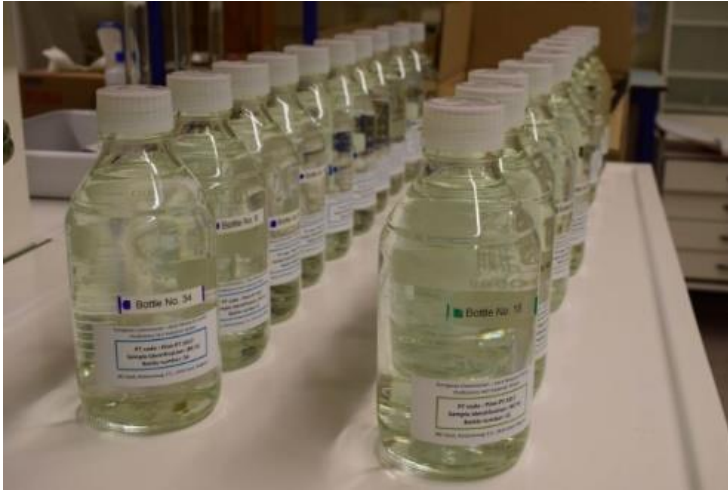
Figure 5. Bottles with radon in water ready to be shipped to monitoring laboratories. Source:JRC.
