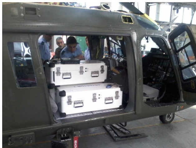
Figure 2. AGS equipment mounted in an Agusta helicopter. The detectors are in the bottom cases, the electronics are in the top case.
